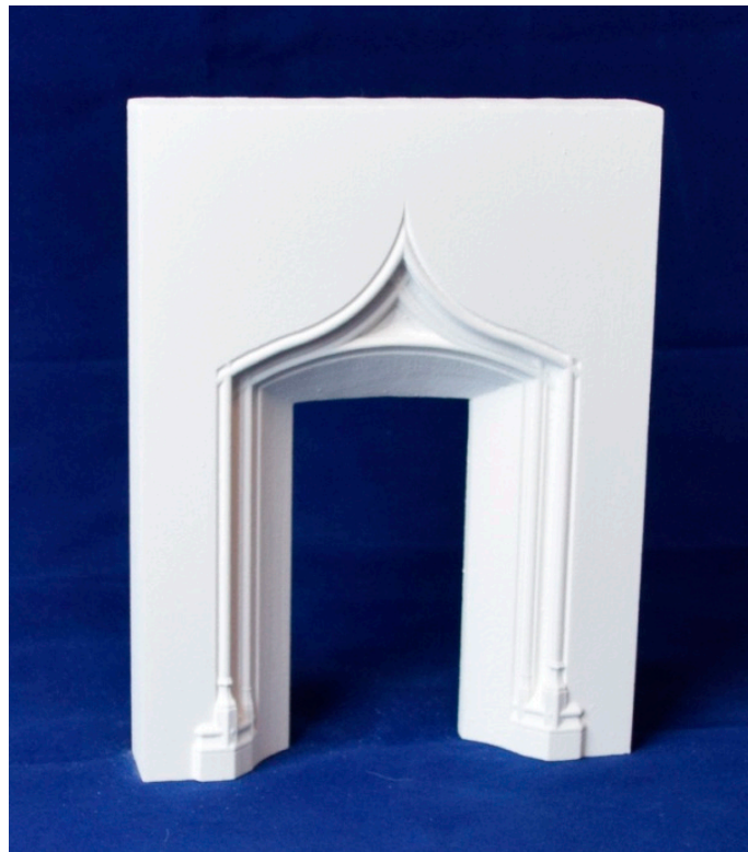
Figure 16. Model of Portal No. 28. Technic: powder printing (3DP). Printing with Z Printer 310 (Z Corporation, Burlington, MA, USA). Material: zp ® 150 and zb ® 60 binder (Z Corporation, Burlington, MA, USA).
