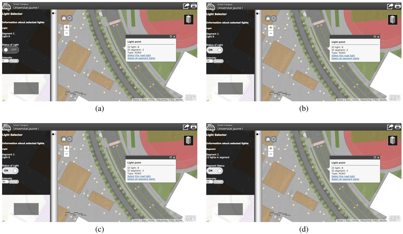
Fig. 7: Desktop Monitoring System: (a) selecting light, (b) switch on a single light, (c) modify light intensity, (d) select multiple lights.
