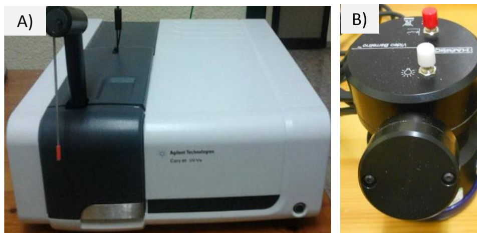
Figure 28. A) Cary 60 Fiber Optic UV-Vis spectrophotometer and B) Remote fiber optic DR accessory.
