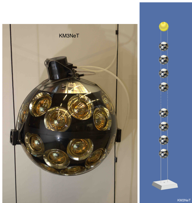
Fig. 2.17.: Left: Picture of a KM3NeT DOM. Right: Example of a KM3NeT DU. Figures obtained from [106].
