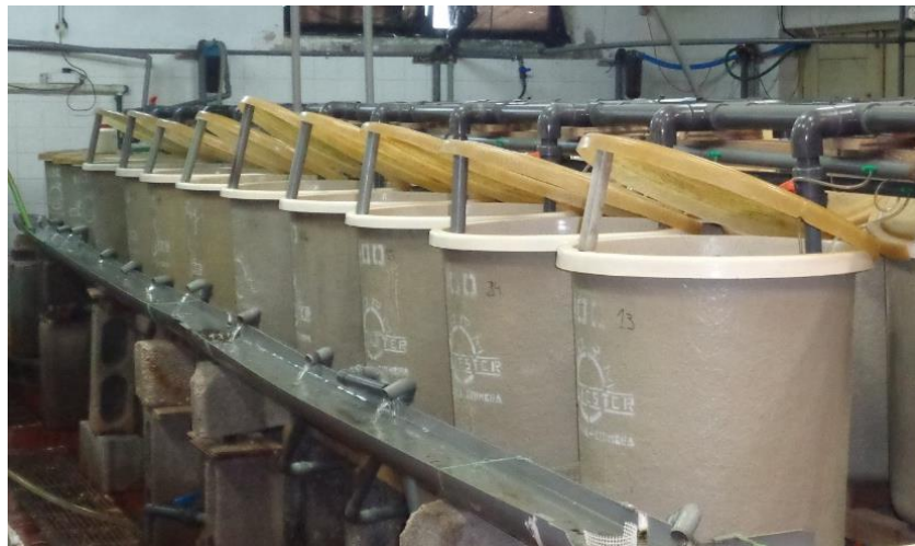
Figure 5. Thermo-regulated recirculation water system
