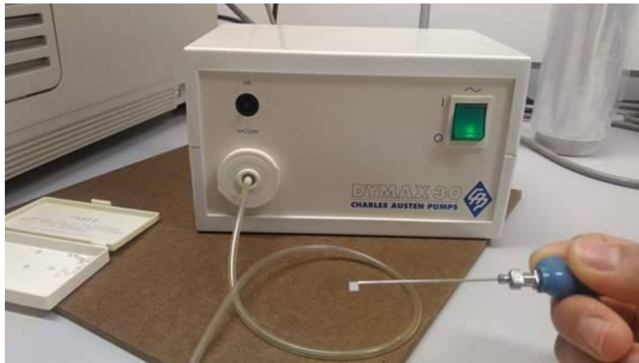
Figure 3.11: DYMAX 30 Charles Austen Pumps Ltd. with Vacuum Tweezer.
