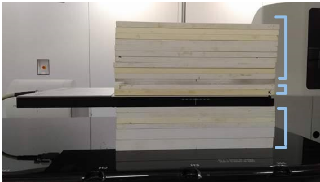
Figure 3.9: Experimental set-up with 20 plates of RW3 phantom, indicated in blue.
