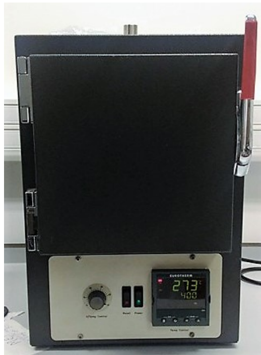
Figure 3.4: The oven of Carbolite® coupled to 3204 Process Controller.
