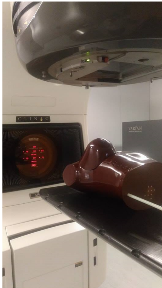
Figure 4.31: Experimental set-up of the Alderson RANDO Phantom irradiation.
