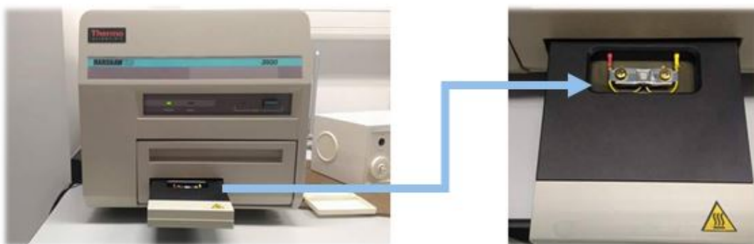
Figure 3.2: The Thermo Scientific™ HARSHAW TLD™ Model 3500 Manual Reader and highlighting planchet provides manual readout of TL chips, disks, rods and cubes in a broad variety of sizes.
