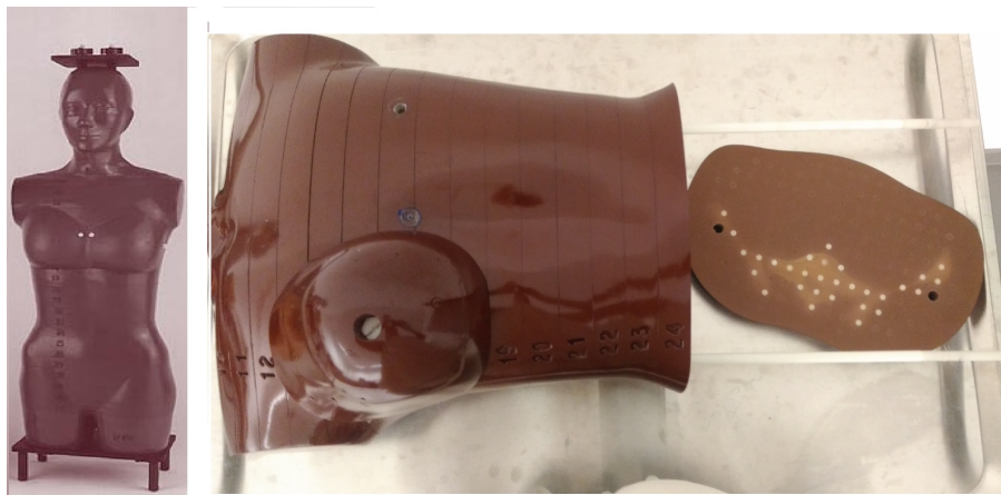
Figure 3.8: Female Alderson Radiation Therapy phantom (ART). [62]
