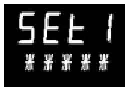
Figure A.2: The upper section of the display shows the set selected, the lower section shows the five digits which make up the set.
