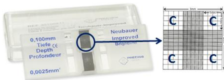
Figure 9 Picture and representation of a Neubauer chamber. The cells on the chamber quadrants represented with “C” are counted.
