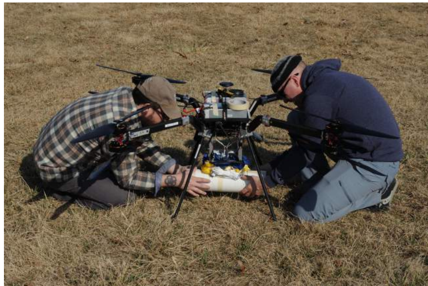
Figure 29: Large UAS with hot wire melter payload release mechanism
