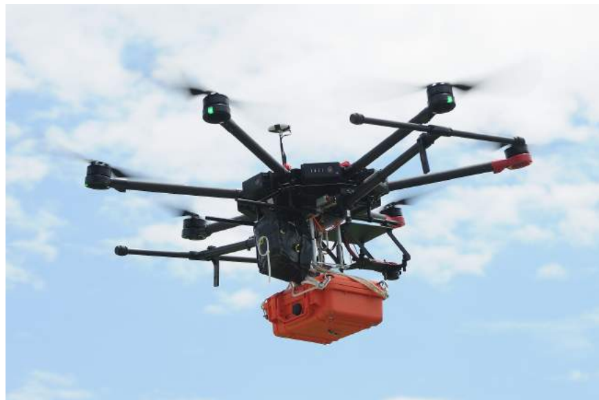
Figure 27: DJI M600 with magnetic parachute release system
