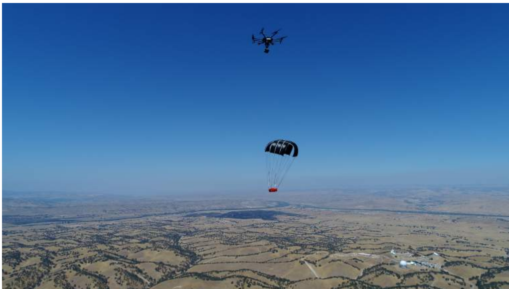
Figure 28: Perfect parachute deployment from M600 UAS with magnetic payload release
