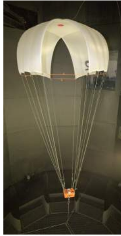
(a) Steerable cruciform system installed in the vertical spin tunnel.
