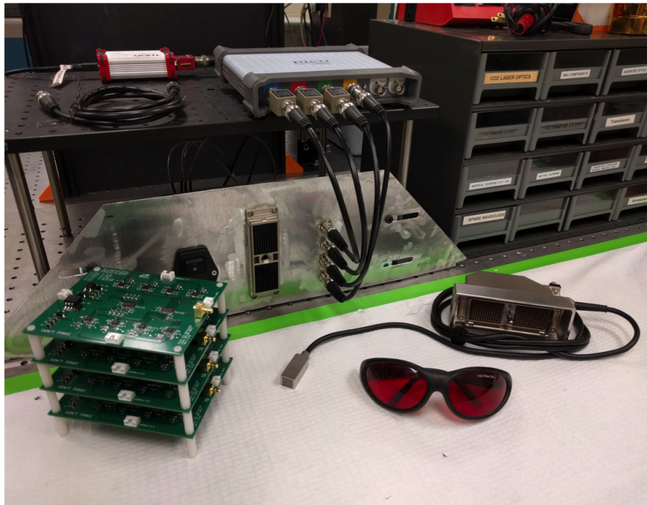
FIGURE 5.8 The assembled multiplexer boards are stacked and fed unregulated \pm 8\text{ V} and ground, 8 signal inputs each, and 3 arduino address signals. The multiplexed signals are output via SMB connectors to BNC front-panel ports, which then feed to the 4 input channels of the Picoscope 5442B, including 50\ \Omega feedthrough terminators on each channel to minimize reflections.
