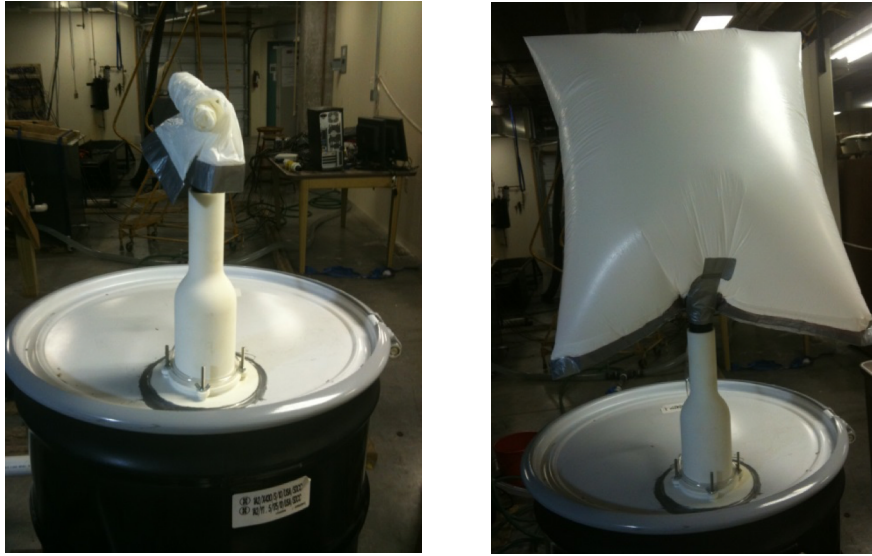
Figure 14 Visual of left empty and right full trash bag for airflow measurement
