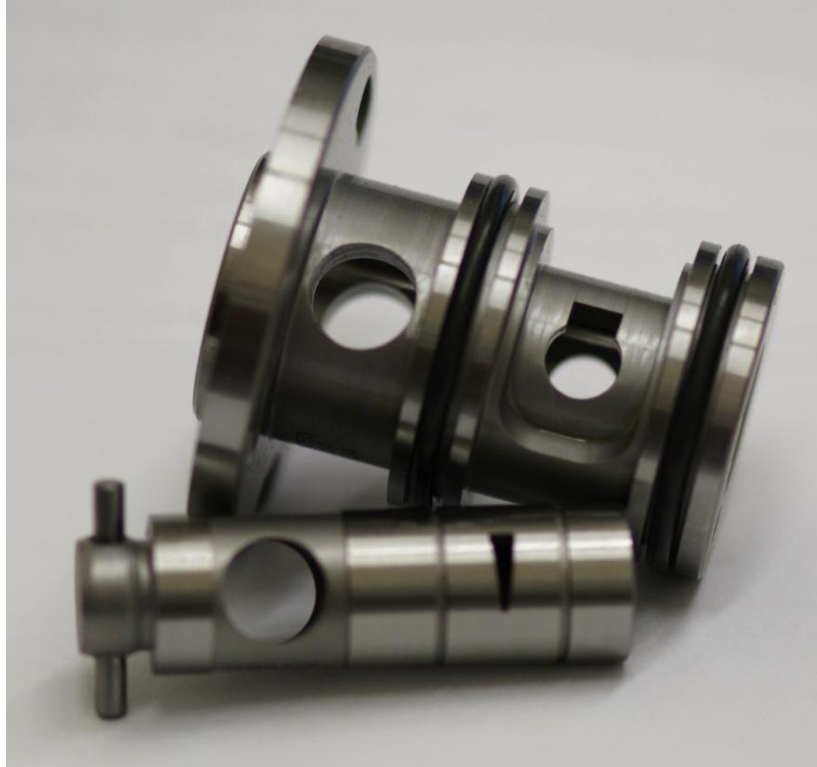
Figure 4.14. IMV disassembled. The dimensions of the triangle portion in the valve are approximately 2.7 mm x 8 mm.
