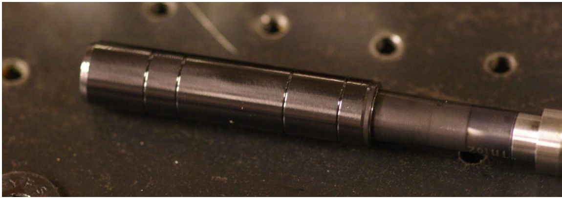
Figure 4.4. Piston side view (length of largest diameter is 59 mm, overall length is 103 mm)
