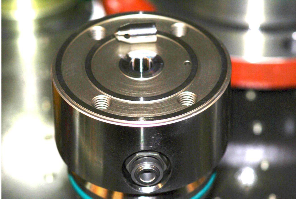
Figure 4.7. Cylinder head with inlet check on the side and discharge check valve placed on top.
