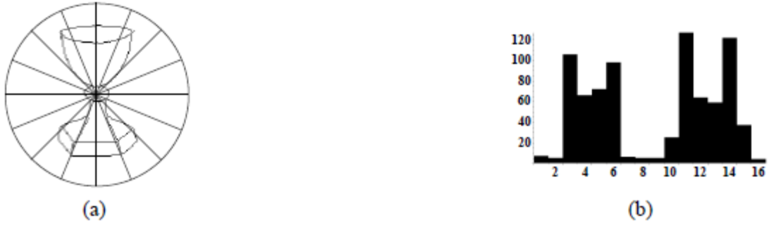
Figure 2.22: Graphical representation of the circular histogram. (a) The center of gravity of the watermark is used as the middle point; (b) The number of pixels present inside a radial segment.
