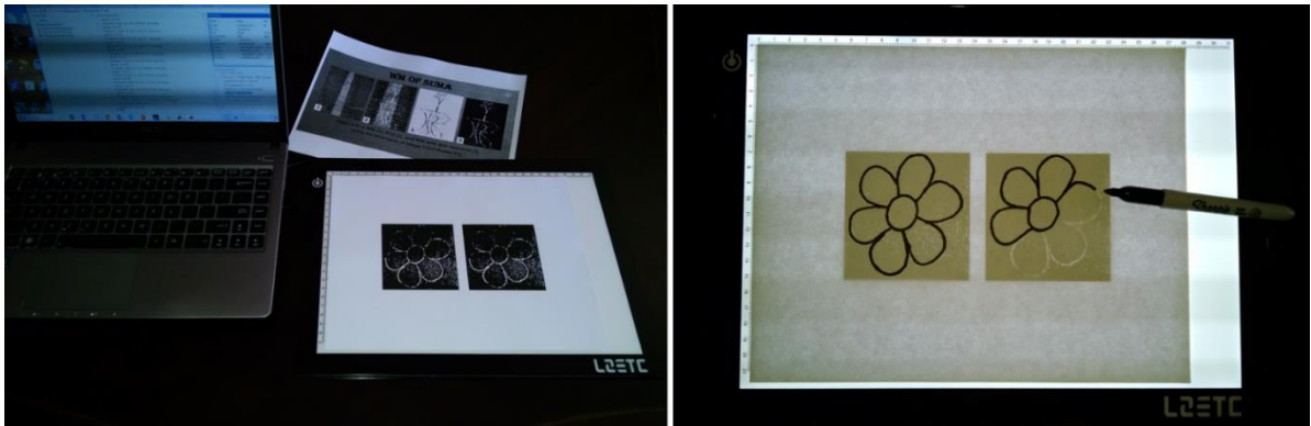
Figure 2.54: LED backlight with the preprocessed image of Fleur a six petals watermarks (left). The tracing is performed with black marker (right).
