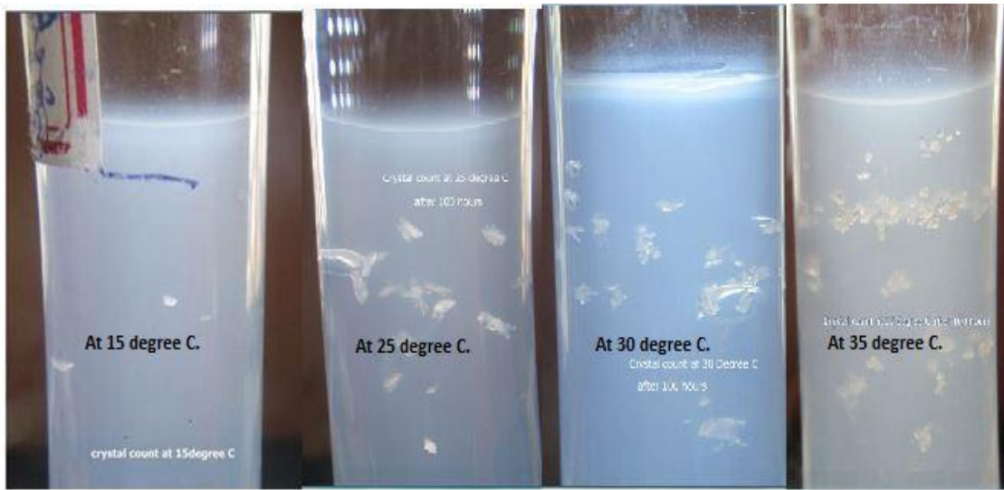
Figure 4.6: Photograph showing increase in nucleation rate with an increase in temperature from left to right.
