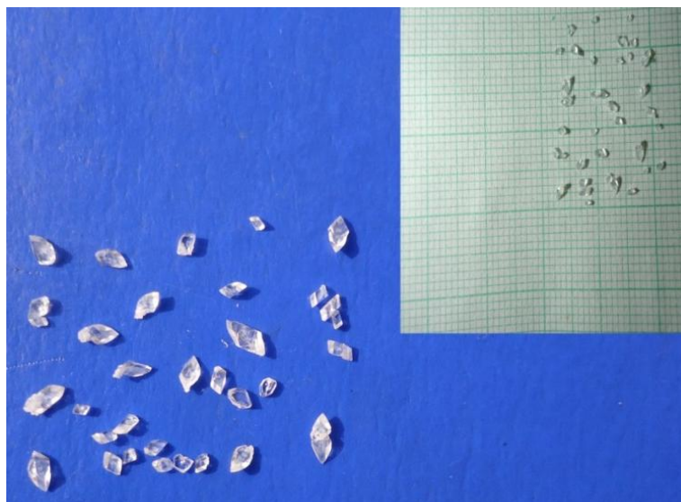
Figure 4.11: Optical micrograph of some typical single crystals of mixed GdTb fumarate.
