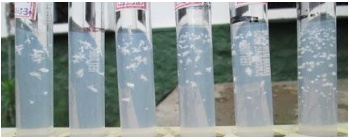
Figure 4.5: Photograph showing increase in nucleation rate with pH in the range 5.0 \leq \text{pH} < 6.0 .
