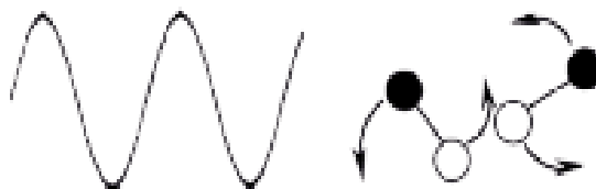
Fig. 2. Dipolar molecules try to align with oscillating electric field of microwaves.
