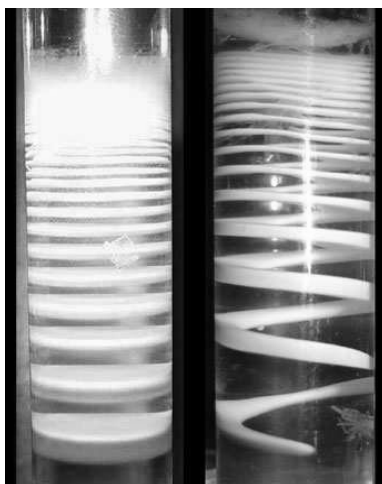
Figure 2.4: Disc and helical Liesegang rings of calcium phosphate in silica gel.
