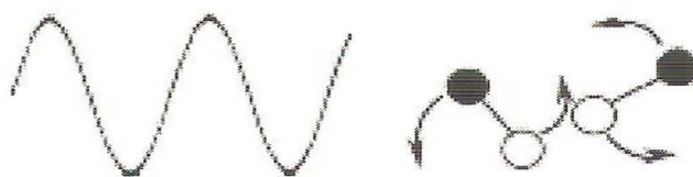
Figure 1.2(a): Dipolar molecules try to align with oscillating field of microwaves.
