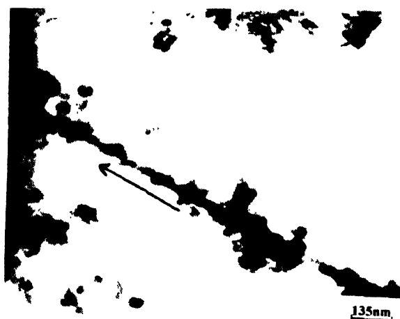
Figure 2(a). Transmission electron micrograph of one dimensional aligned Si nanoparticles of average size as \sim 50 nm. The one dimensional alignment is outlined by arrows. Alignment is upto 800 nm.
