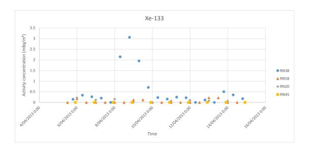
Figure 1: Time series (in UTC) of the observed activity concentrations of Xe-133 that were used in the inverse modelling.
