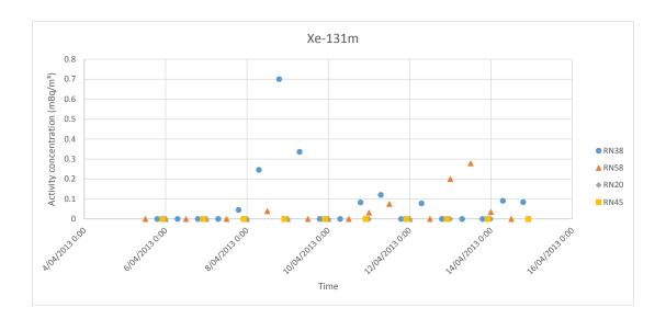
Figure 2: Time series (in UTC) of the observed activity concentrations of Xe-131m that were used in the inverse modelling.
