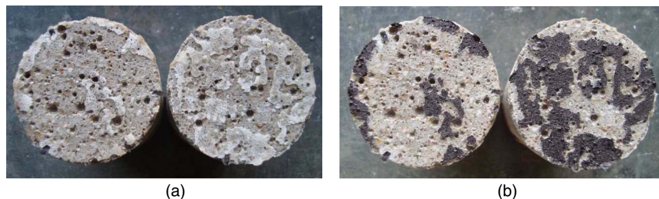
Fig. 3. Polyurethane on the crack surface: (a) after performance of an axial tensile test; and (b) after the polyurethane was colored with a black marker.
