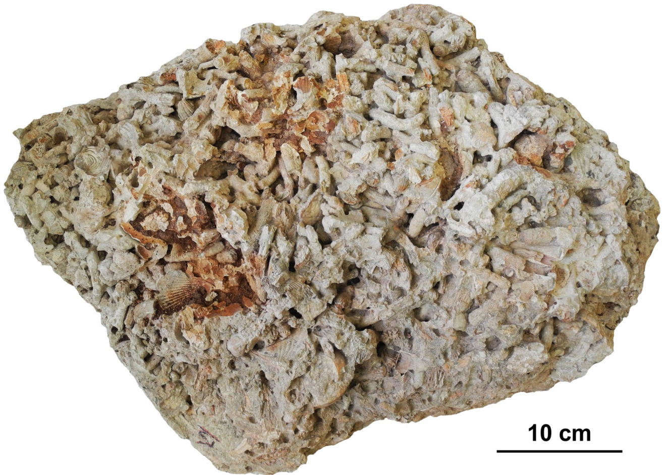
Fig. 4 One of the large samples of Aturia level collected for laboratory analyses. The block has been placed upside down to show the macrofossil accumulation that constitutes the basal coral rudstone facies
