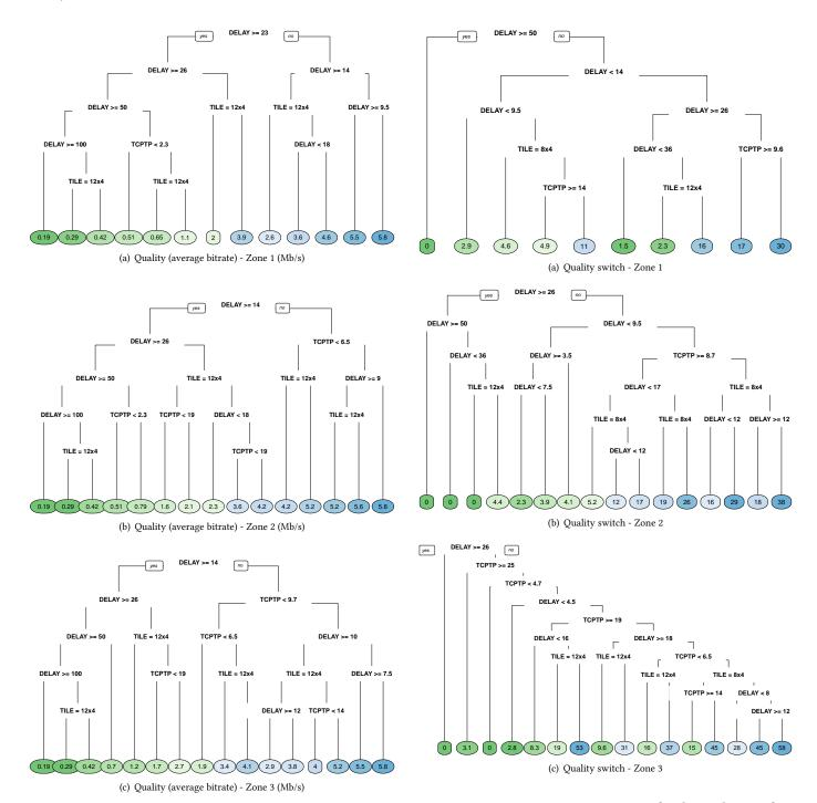
Figure 7: Regression tree representation for the predictors of the VR playout performance metric: quality. Leaf node colors go from dark green (for the lowest value for the predicted variable) to dark blue (the highest predicted value).
