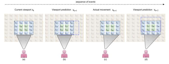
Figure 1: Example of the working principles of the viewport prediction.
