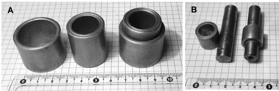
Figure 3: Examined types of joints: A – “bush-on-bush”; B – “bush-on-rod”
