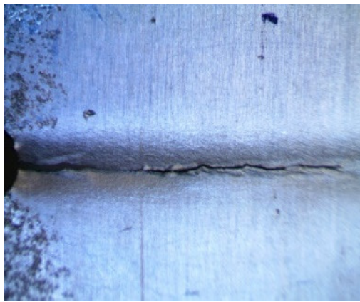
a) The initial crack, 25mm in length
