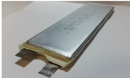
Figure 6.5. 8048168C Lithium Ion Cobalt Oxide (LCO) Polymer Battery.
