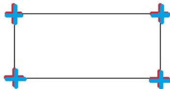
Fig. 2.1 The registered image with 4 blue “+” marks overlapping the reference image with 4 red “+” marks.
