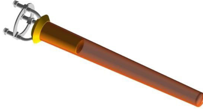
Figure 2.16: The g_{11a} 40-cm-long, 4-cm-diameter target cell, constructed in a truncated conical design from kapton.
