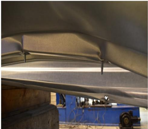
Figure 36. Condition of 0.85mm Sheet at ultimate load (Setup-2)
