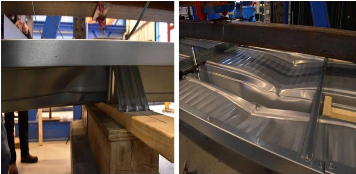
Figure 41. Buckling of section over mid-support and mid-span (1mm Setup-1)
