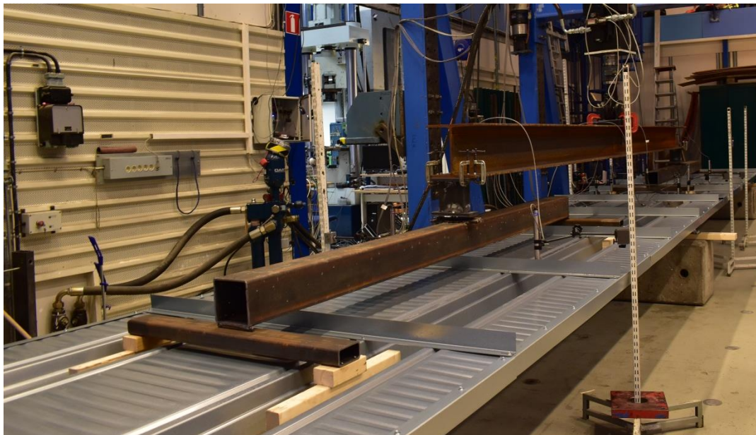
Figure 27. Loading Mechanism in Experimental Setup
