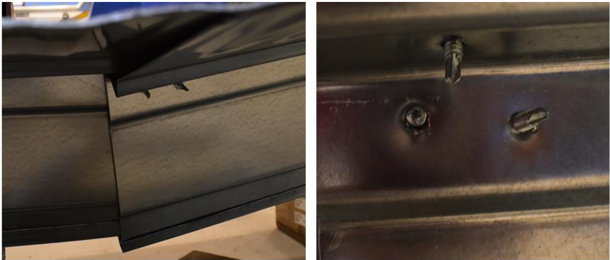
Figure 57. Condition of Hinge at ultimate load (1.5mm Setup-2)
