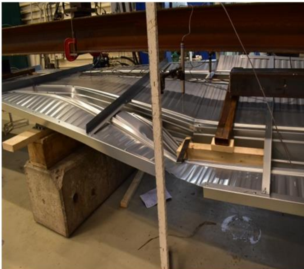
Figure 37. Buckling of 0.85mm Sheet at ultimate load
