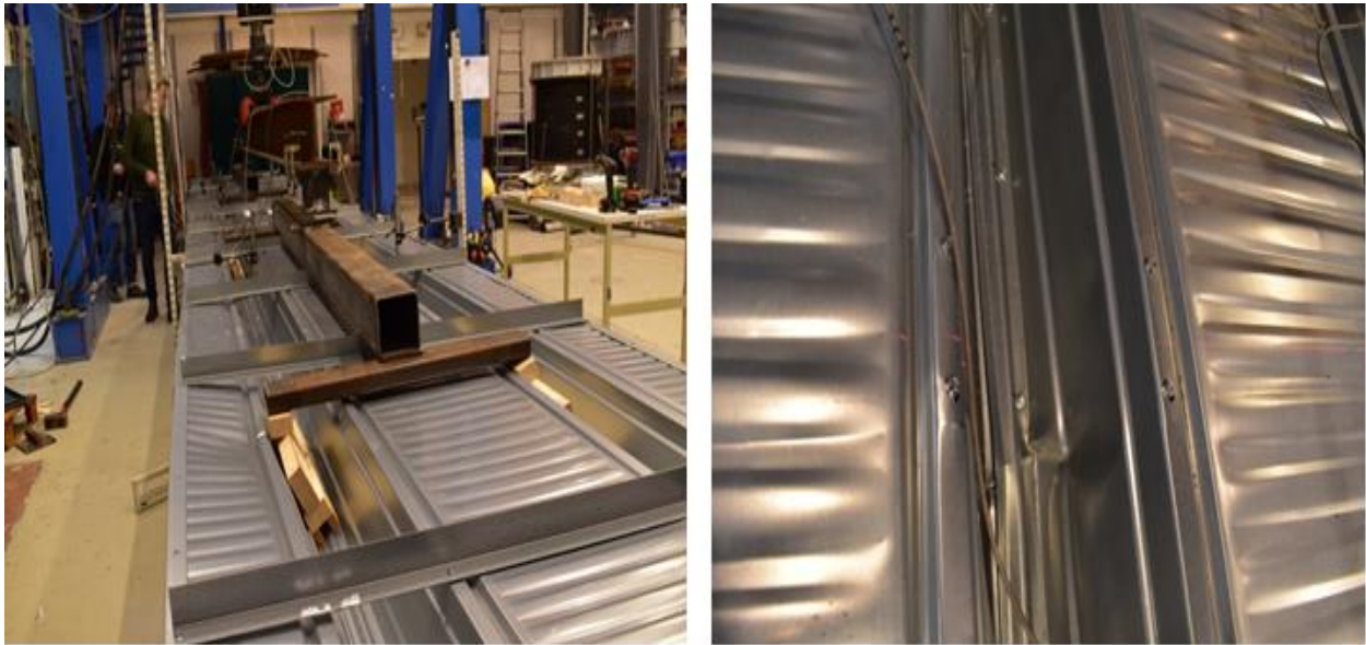
Figure 31. Tilting of loads and condition of internal support at collapse
