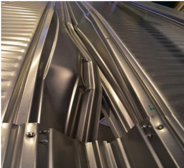
Figure 36. Condition of 0.85mm Sheet at ultimate load (Setup-2)
