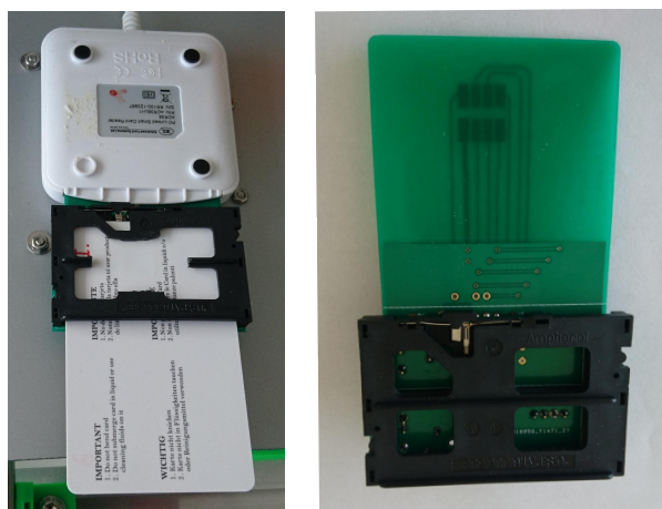
Figure 7.2: Measuring adapter with plastic part and with the part cut out
