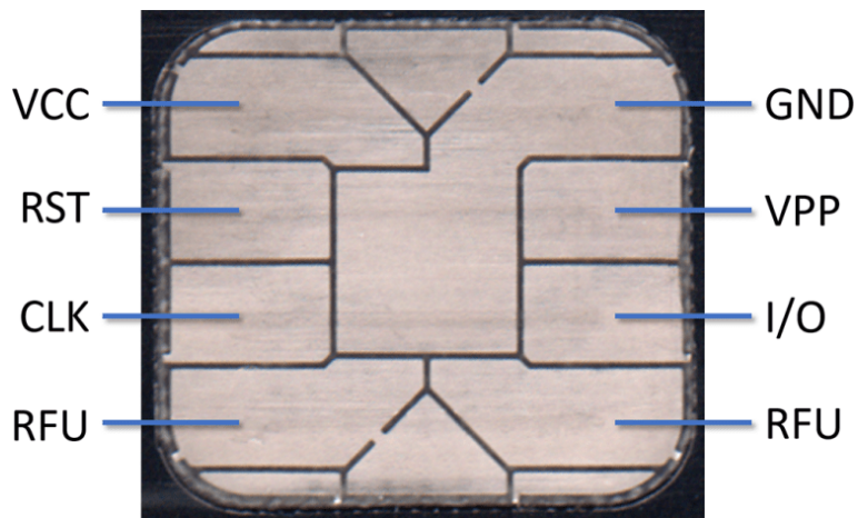
Figure 4.10: Contact smart card PINs [3]
