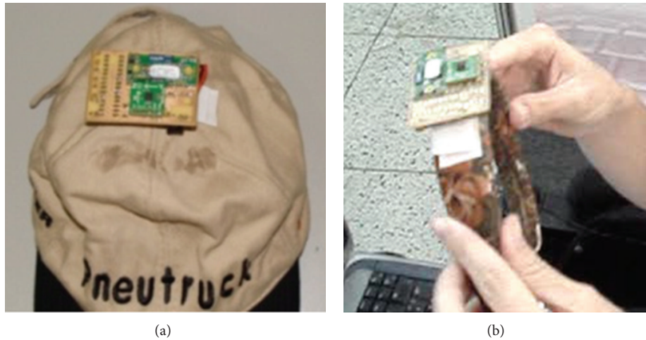
FIGURE 4: Inertial sensor mounted on a cap or headband. These two accessories were proposed to provide comfort to the user's tastes.
