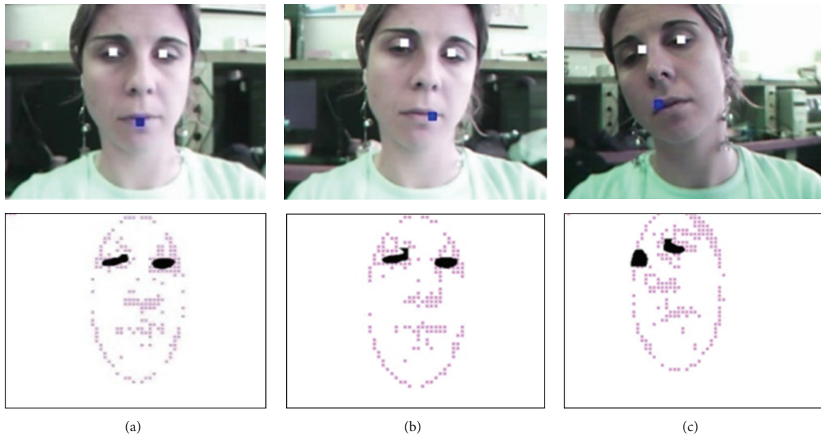
FIGURE 3: Examples of the facial characteristics detection. Three cases of eyes detection are shown, these case are (a) centred head, (b) head's left-move, and (c) head's right-move.
