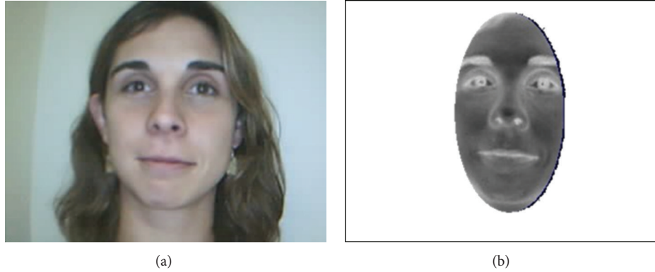
FIGURE 2: Vision based interface. (a) Image obtained by the webcam interface at a resolution of 320 \times 240 pixels. (b) Ellipse ROI image obtained after the skin detection (in YCbCr space) and the ellipse calculation.
