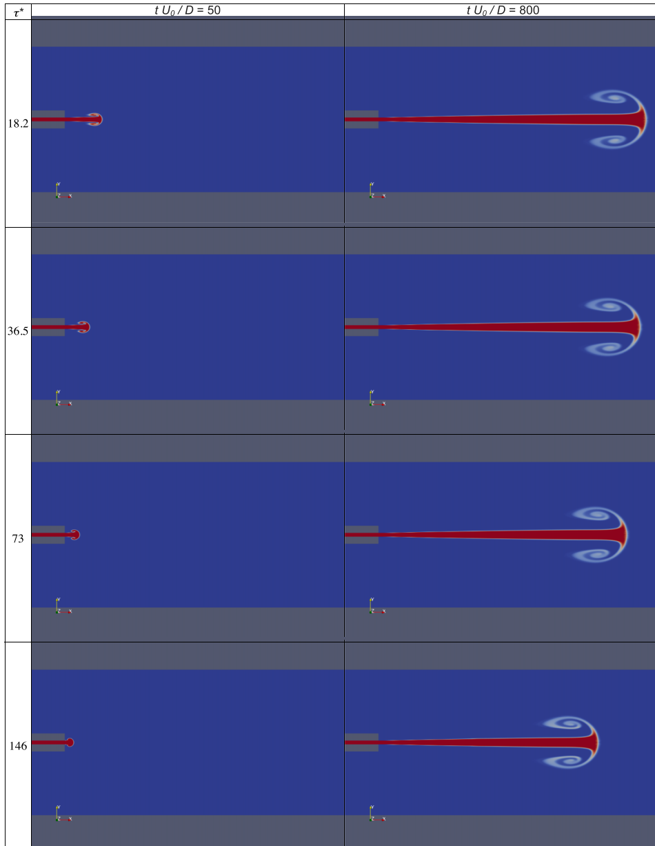
FIG. 25. 2D Numerical simulations to illustrate effect of time constant \tau of the velocity ramp. Tracer concentration at Re = 73 . Left column: tU_0/D = 50 , right column: tU_0/D = 800 . From top to bottom, \tau U_0/D = 18.25 , 36.5, 73, and 146.
