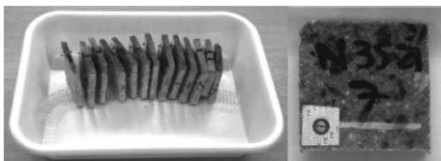
Figure 1. Samples for water sorption and resistivity determination of unsaturated concrete
