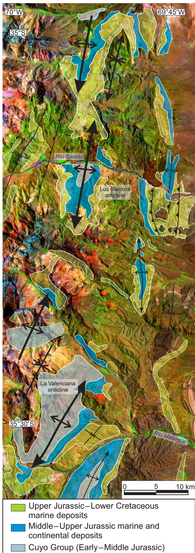
Figure 14. Belt of anticlines interpreted in this work as the result of the inversion of Mesozoic half-grabens. Folds follow the orientations of the main normal faults of the Neuquén Basin.
