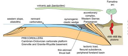
Figure 11. Diagrammatic cross section of tectonic model for the Middle–Late Ordovician foreland basin and clastic wedge in the context of accretion of the Precordillera to Gondwana and the Oclovic orogeny.
