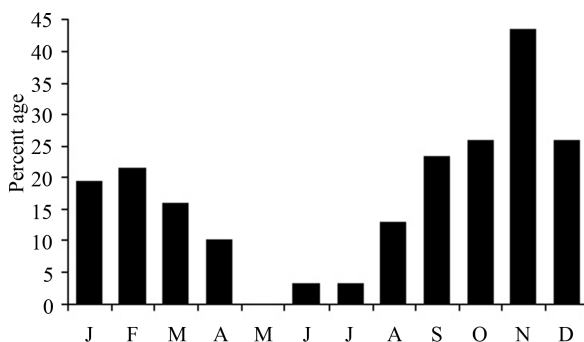
Figure 2. Wind frequencies (in percentage) with velocities over 22 km/hour.
