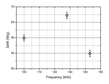
**Figure 3**: SAR values in SiOx- $Fe_3O_4$  aqueous suspensions vs. driven field frequency at a fixed field amplitude of 20.3 kA/m.
