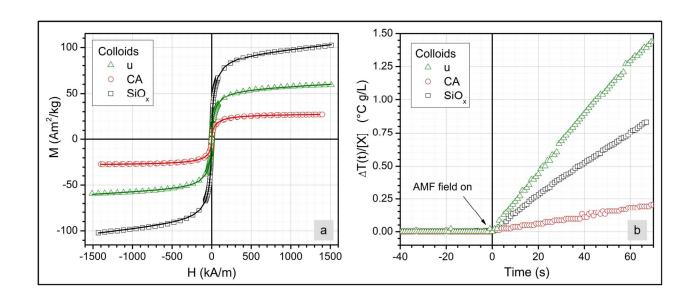
**Figure 2**: a) Room temperature specific magnetization (M) *vs.* applied field (H) loops recorded with VMS- dc magnetometry, data was normalized by mass of Fe<sub>3</sub>O<sub>4</sub>. b) Heating curves of MNPs aqueous suspensions measured at 128 kHz and 20.3 kA/m. Data is plotted as temperature increase  $\Delta T$  scaled with concentration [x] vs. time.
