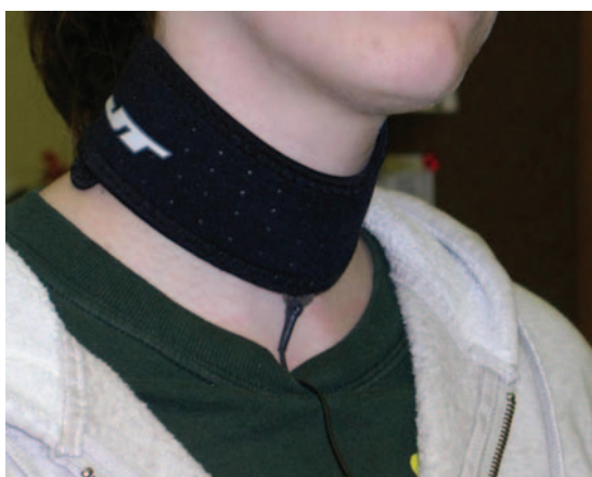
Fig. 2. Swallowing sensor: a miniature throat microphone was glued to a neoprene collar that was fastened to the neck of the subject using flexible velcro. Microphone was located over the laryngopharynx.
