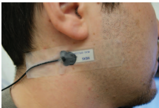
Fig. 1. Chewing sensor: a piezoelectric film strain sensor was attached immediately below the earlobe and above the gonial region of the mandible using medical tape.
