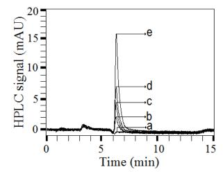
**Fig. 3:** Chromatographic elusion of MDA-TBA<sub>2</sub> condensation product at different column temperatures assayed during the optimization of HPLC conditions to determine MDA in cryopreserved bovine samples.
