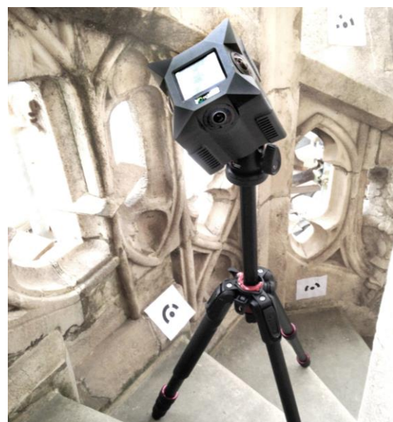
Figure 1. NCTech iSTAR during the surveying operations.
