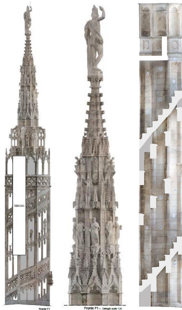
Figure 5. Orthoimages of the Amadeo Spire: the complete (left) and a zoom of the top portion (centre) of the outside elevation. On the right, the inside elevation obtained with monocular photogrammetric network performed with Nikon D810 and 12mm fisheye lens.
