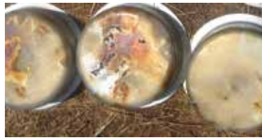
Pots after cooking for 3 hours with (a) briquettes, (b) charcoal and (c) kerosene.
