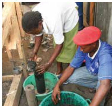
(a) Charcoal briquettes moulding in recycled plastic containers and (b) compacted in wooden manual press and (c) sawdust briquettes compacted using metal manual press. All photos by Mary Njenga
