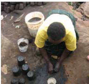
(a) Charcoal briquettes moulding in recycled plastic containers and (b) compacted in wooden manual press and (c) sawdust briquettes compacted using metal manual press. All photos by Mary Njenga
