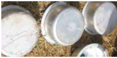
Pots after cooking for 3 hours with (a) briquettes, (b) charcoal and (c) kerosene.
