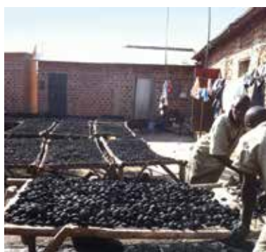
(a) Drying briquettes on beds in Kampala (b) and on rooftops in Nairobi
