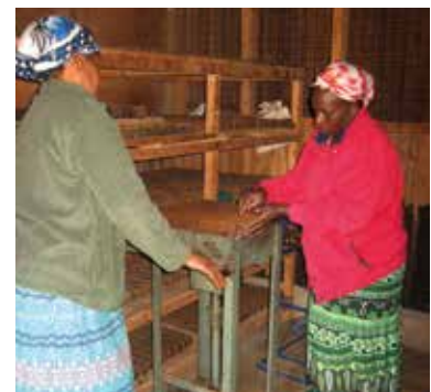
(a) Charcoal briquettes moulding in recycled plastic containers and (b) compacted in wooden manual press and (c) sawdust briquettes compacted using metal manual press. All photos by Mary Njenga
