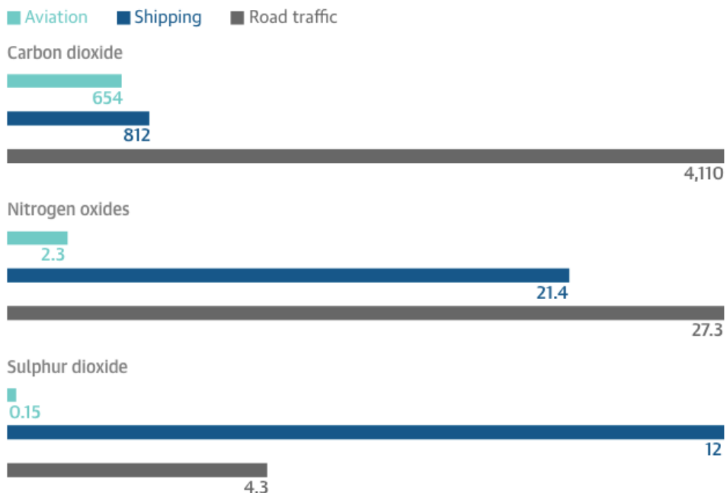
Figure 2.1: Annual emissions in million tonnes (differing scales). Source: Institute of Atmospheric Physics (DLR) (March 2007) Comparing fuel consumption, CO 2 and other emissions from international shipping and craft.
