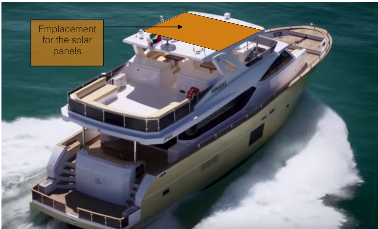
Figure 8.1: Schema about solar panels disposition. Source: photo from Gulf Craft.
