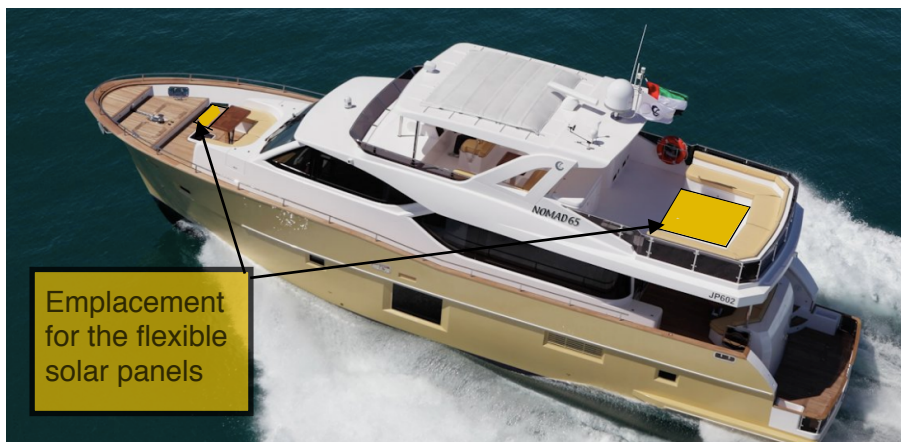
Figure 8.2: Schema about flexible solar panels disposition. Source: photo from Gulf Craft.
