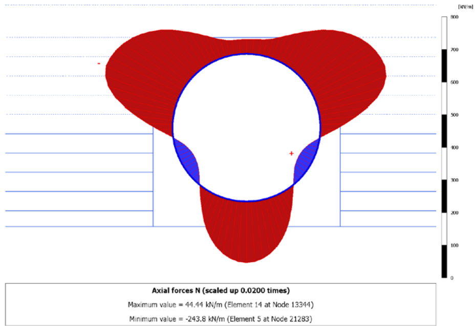
Figure 14. Tunnel lining ring rotation: 0 degrees. Trencher centered load. Symmetric excavation. Axial forces (tensile forces in blue and positive).
