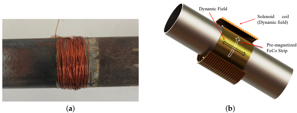
Figure 2. Magnetostrictive transducer used in the test bench. (a) Picture of the transducer and (b) Schematic representation of the magnetostrictive strip and the coil.
