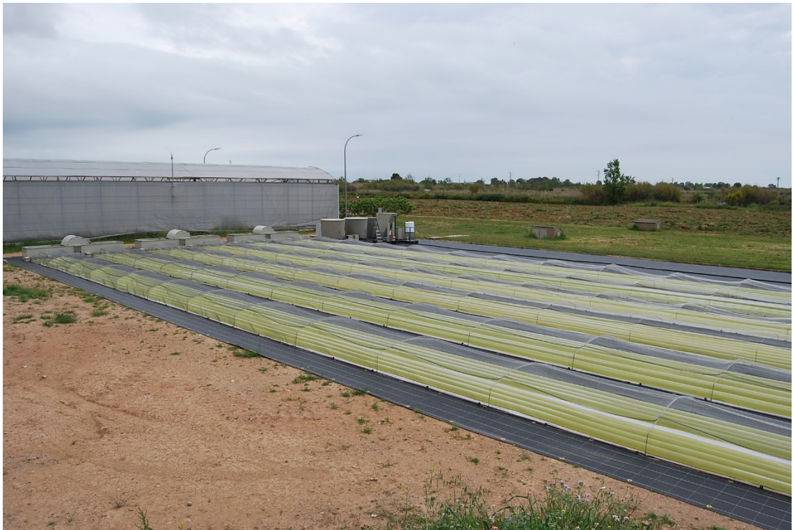
Figure 2. Scheme of one photobioreactor and picture of the experimental plant with the three photobioreactors installed and operating.
