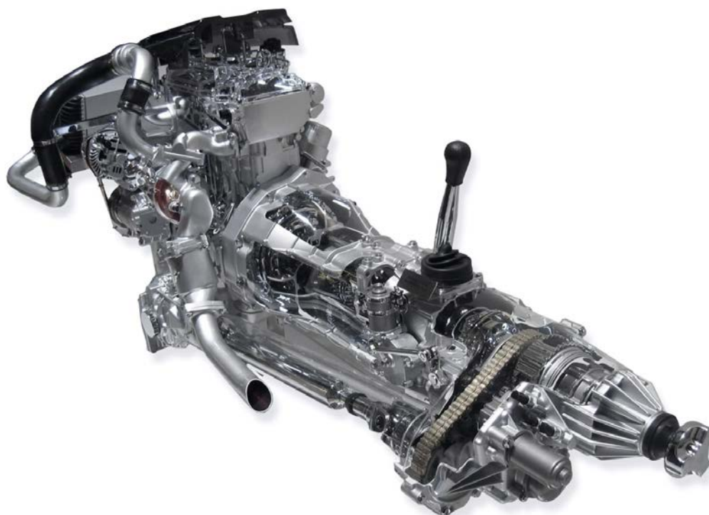
Fig. 1. Nissan Pathfinder Engine. Characteristics: (i) 747 parts and 330 references, (ii) 378 elemental assembly tasks grouped in 140 production line tasks.
