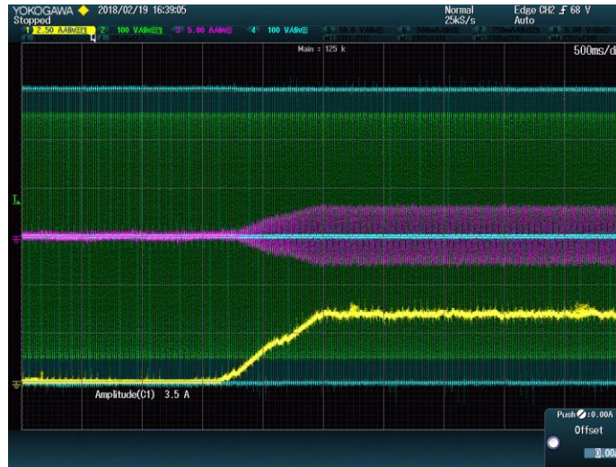
Figure 4.28: System response to MPPT algorithm sampling at 10 kHz. Line-to-line inverter voltage (blue), AC current phase A (purple), grid line-to-line voltage (green), Boost inductance current (yellow) (500 ms/div).
