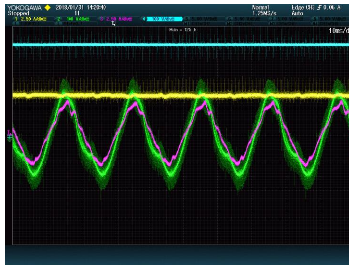
Figure 4.31: System response to MPPT algorithm sampling at 5 kHz. DC-link voltage (blue), AC current phase A (purple), AC line-to-neutral voltage (green), Boost inductance current (yellow) (10 ms/div).
