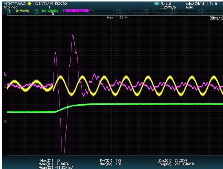
Figure 4.17: Inrush current caused by a 20 VAC step. DC-link voltage (green), AC current phase A (purple), AC line-to-line voltage (yellow) (20ms/div).
