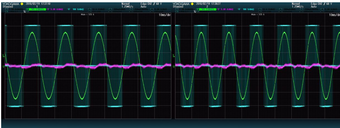
Figure 4.18: PLL synchronization at 50Hz (left) and 60 Hz (right). Line-to-line inverter voltage (blue), line-to-line grid voltage (green), and AC current phase A (purple) (10ms/div).
