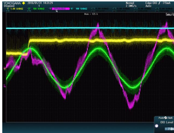
Figure 4.26: 1 A step at boost inductance current reference at 5 kHz. DC-link voltage (blue), AC current phase A (purple), AC line-to-neutral voltage (green), Boost inductance current (yellow) (5ms/div).
