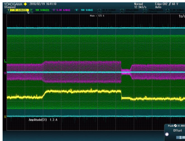
Figure 4.29: MPPT algorithm under irradiance steps, sampling at 10 kHz. Line-to-line inverter voltage (blue), AC current phase A (purple), grid line-to-line voltage (green), Boost inductance current (yellow) (1 s/div).
