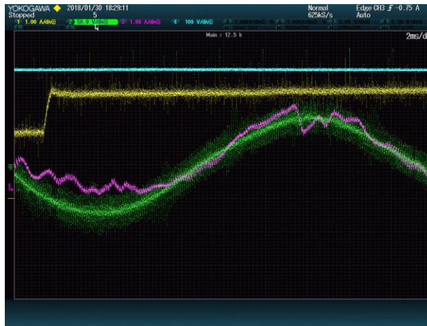
Figure 4.25: 1 A step at boost inductance current reference at 10 kHz. DC-link voltage (blue), AC current phase A (purple), AC line-to-neutral voltage (green), Boost inductance current (yellow) (2ms/div).
