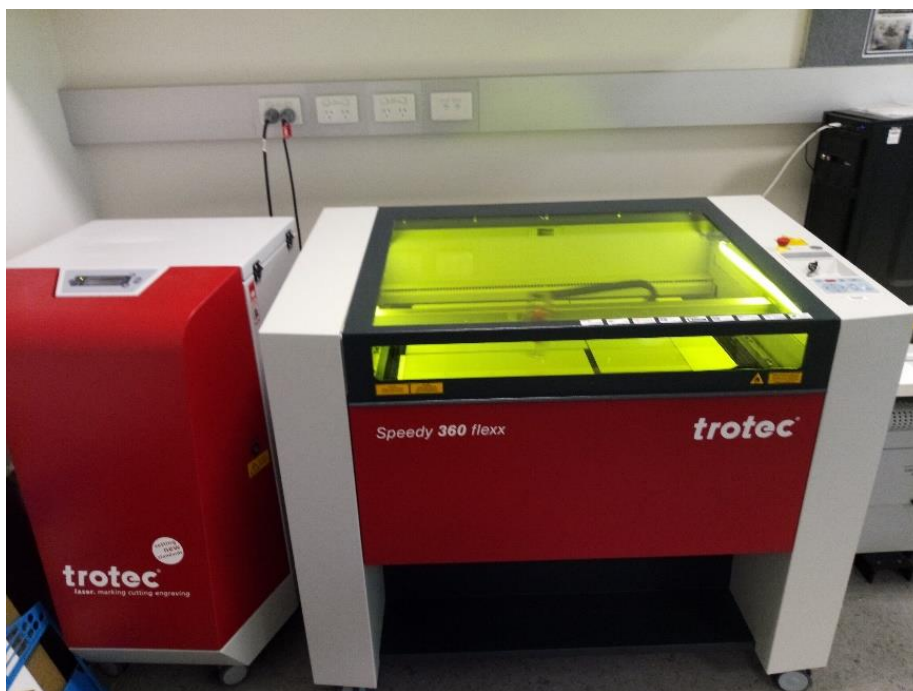
Figure 6 – Laser cutter/engraving system used for etching RuO 2 , manufacturing acrylic-wells and stencils.
