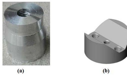
Figure 3-26. (a) A workpiece with one machine surface and one tap [187], (b) a workpiece with one machined surface and two taps in the same size [188].
