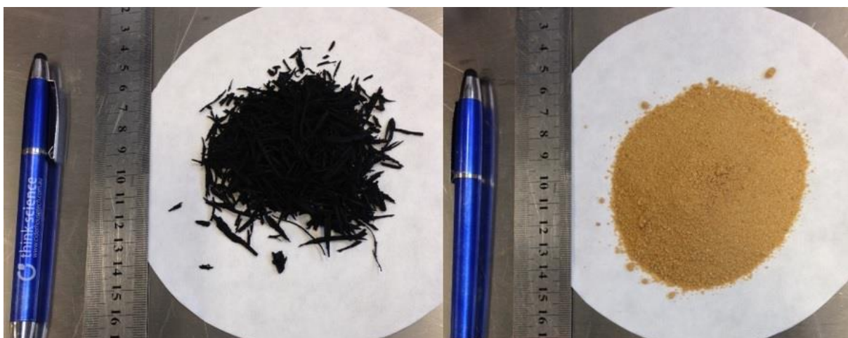
Fig. 3.1. Materials used: tyre fibres; sandy soil
