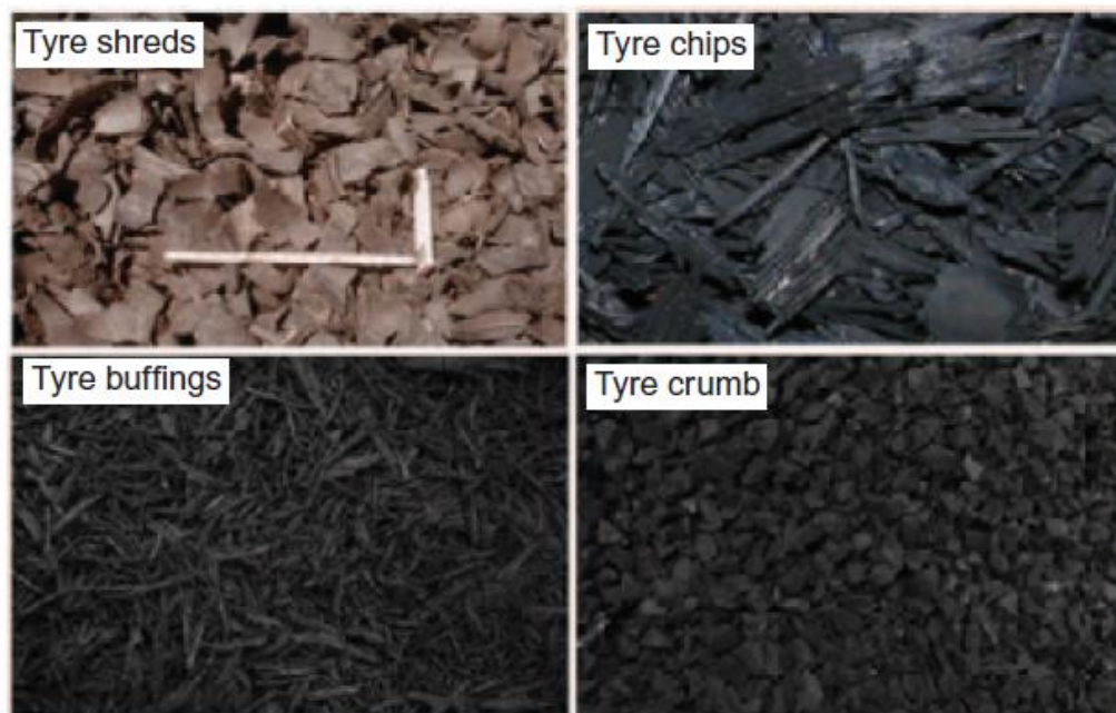
Fig. 1.2. Different processed tyre waste types (Edinçliler et al., 2010)
