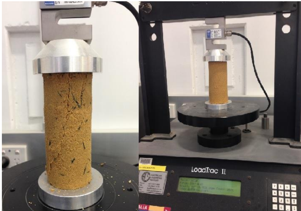
Fig. 3.4. The unconfined compression test equipment; the specimen with cement and tyre fibre content; automatic loading machine
