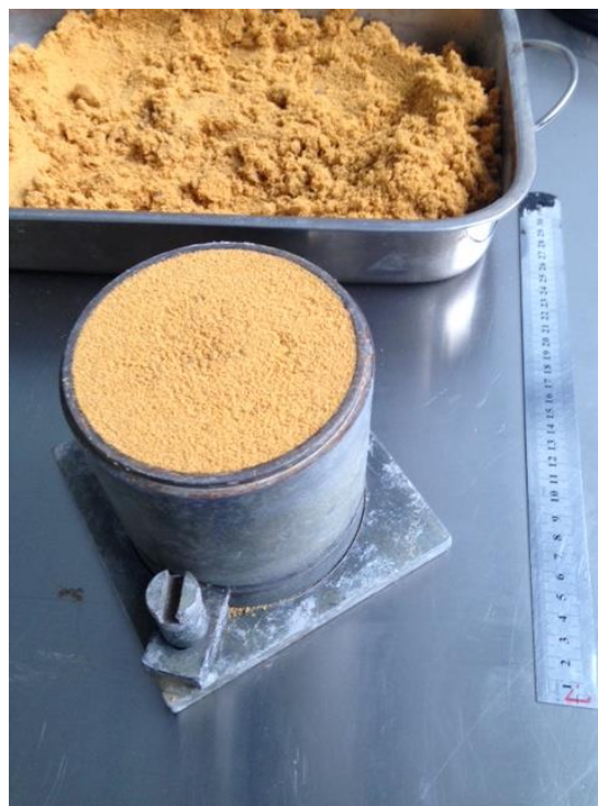
Fig. 3.3. Compaction mould with compacted sample
