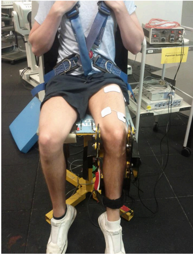
Figure 2. Participants were firmly strapped into the rigid seat across across the hips and chest, with the leg secured above the ankle. Three adhesive neuromuscular electrical stimulation electrodes were placed over the thigh (see text for details).
