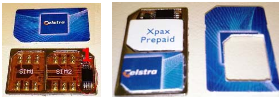
Figure 26: Hyper-Card and Telstra SIM card before and after SIM cutting and placement with another SIM card.
